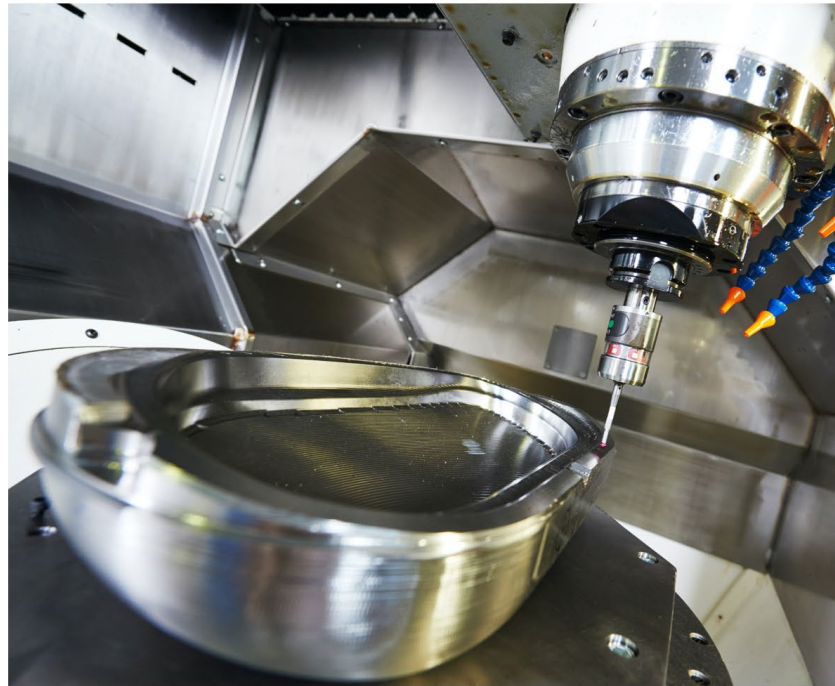
Capturing metrology data on machine tools where parts are made creates a singular opportunity to identify machine-based changes as they occur and adjust them in real time.
